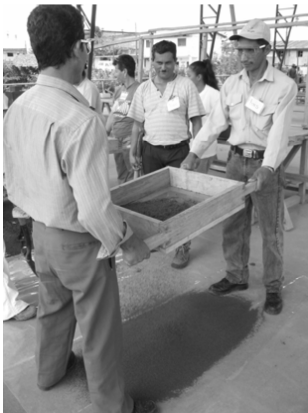
Preparation of sand media as part of CAWST training workshop, Ecuador
